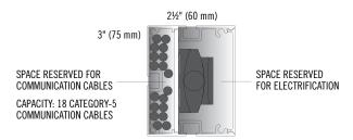
• When specifying, it is recommended to order a raceway in the size immediately smaller than the dimension of the furniture it will be installed on (for example: DT2472 + EC2RACE60) in order to allow space for exteriors, enable cables to round a corner, or any other reason.
